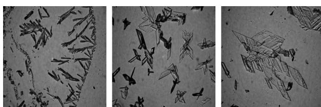
Fig. 2. Crystals of SPA grown for 30 minutes (magnification 200x): from left to right at 23 °C, 30 °C, 37 °C
